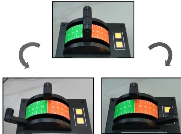
8. Move the left throttle lever to the forward maximum. And to the backward maximum.
