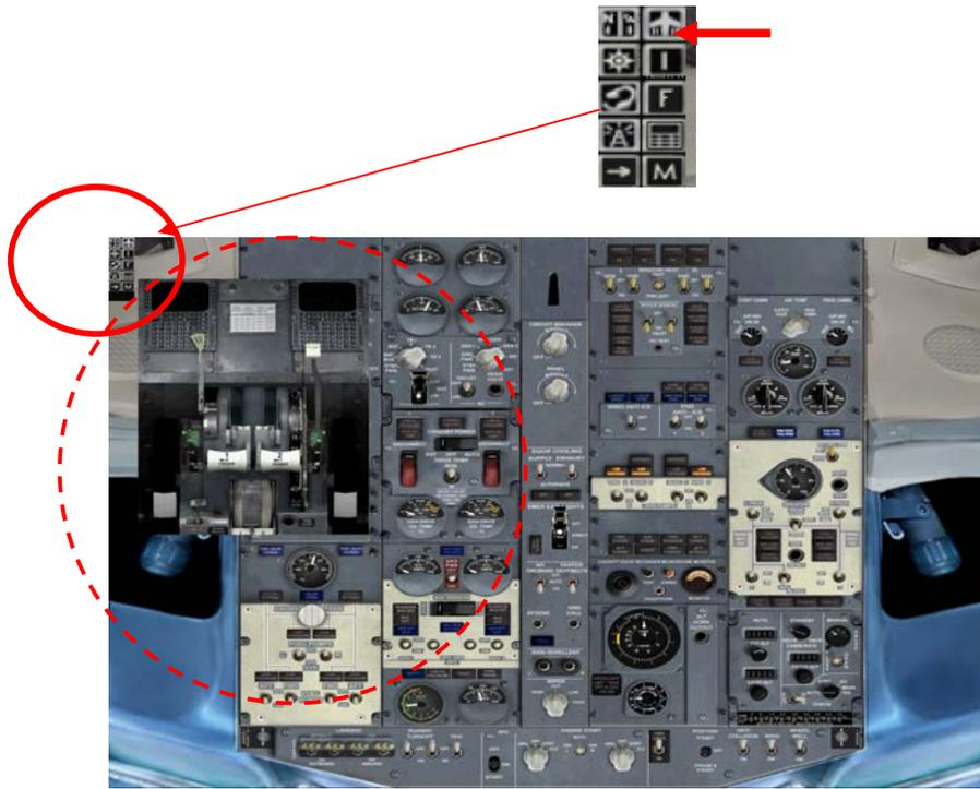
As you can see the throttle is in **idle** make sure that your joy stick also is in the idle position. On the lower part of the overhead is the engine start. Its normal to start Engine Right to Left (don't ask me why) so turn the knob of Right engine to GND and you will hear engine spooling.
