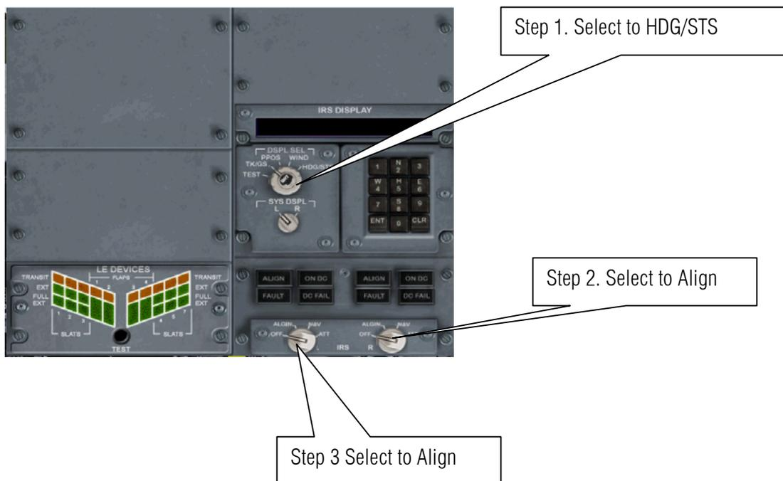
34. The number on the IRS display is 3 means 3 minutes.
