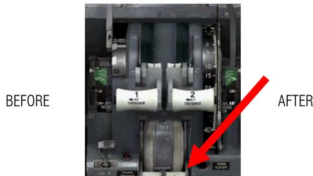
25. As you can see the knob comes back to OFF position. Now start the Left Engine by clicking the knob of Engine Start to GND.
