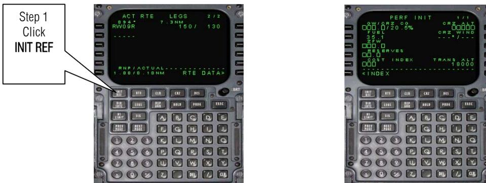
52. Using the CDU numeric key pad enter the following: On 1L enter 150. On 1R enter 10000. On 4L enter 6. On 5L enter 80.
