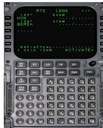
VI. Then type in the remaining way point. Using CDU key pad type **COWLY** and press **3L**. Using CDU and press to **4L**.
