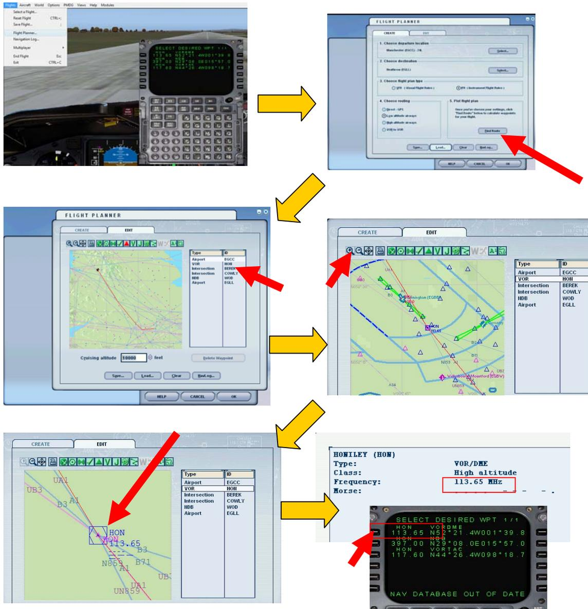
V. Click 1 R Now if have not. Using CDU key pad Type **BEREK** and click **2R**. Just like **HON, BEREK** also have a duplicate Waypoint. This time the way point is not a DME/VOR so just like preceding step open the flight planner and click **BEREK** and check the coordinates. Just like before it's the first one. Then its **1L** again.
