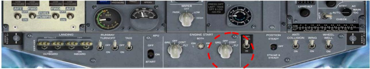
Just like right engine it as you hear its running wait for 10 seconds before clicking the lever of Left Engine on the throttle control to IDLE.
