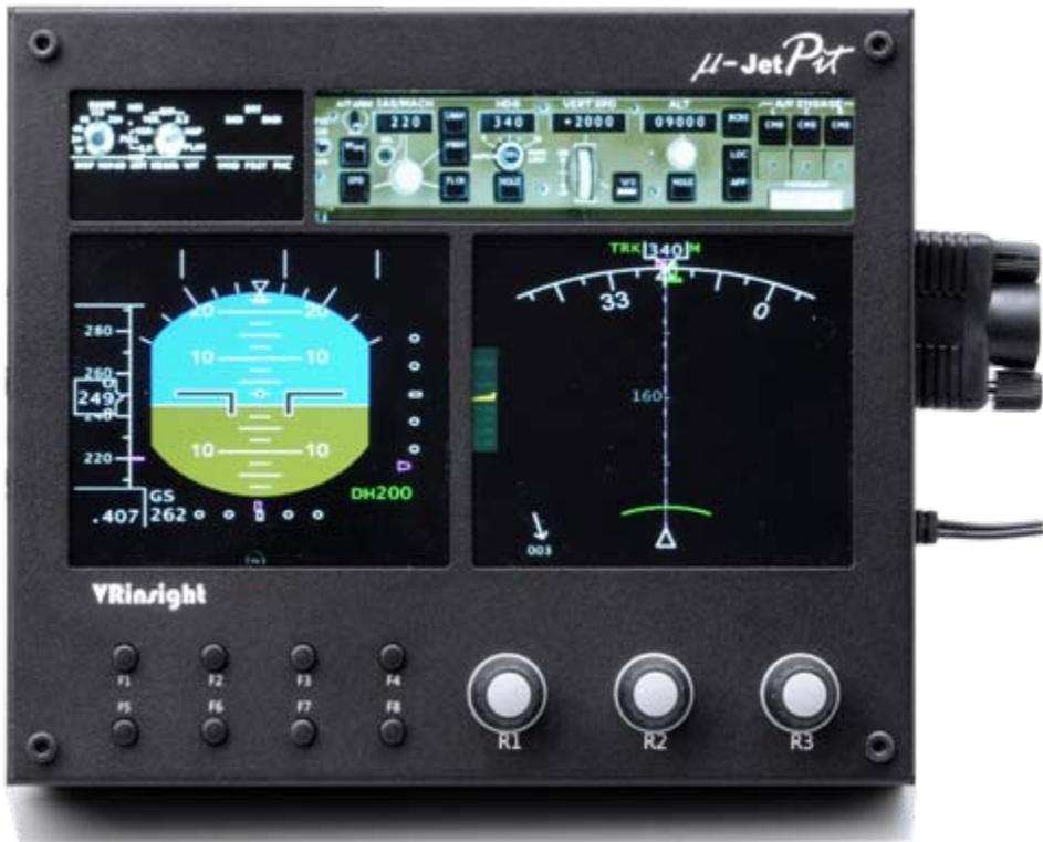
The *μ-JetPit* of VRinsight is a portable instrument panel for jet aircraft. It features a ND, PFD, EFIS and MCP as well as real knobs. All the instruments, buttons and knobs are synchronized with default Flight Simulator jet aircraft and most aircraft add-ons.
