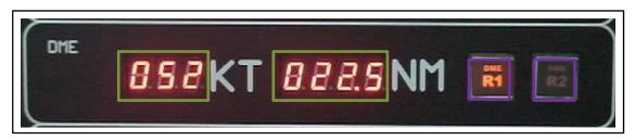
DME Unit: 2 luminous tact switches. 3 digit / 7-segments and 4 Digit / 7-segments displaying the speed of the airplane and the distance between airplane and VOR
