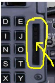
CDU panel is available only FMC/CDU window is opened. After shutting down FMC/CDU window, it works as Hot-Keys. For instance, pressing L1 is same as Pressing F1(L2=F2).
