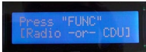
CDU panel supports various aircrafts (MSFS's original aircrafts and other payware aircrafts such as Wilco, PMDG, Level-D & PSS). All of buttons on the panel are user programmable. Use key-mapping software provided; "CDU Key Mapper" for CDU panel. After an aircraft selected, press "Load FS Module" button.
