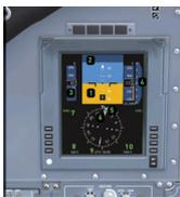
This screen displays the most important information for flying, which is why it is called the Primary Flight Display. The top part shows the AHI (Artificial Horizon Indicator) 1, with the Flight Mode annunciator (FMA) on the top 2, which displays the autopilot modes, the AIRSPEED is on the left 3 and the ALTITUDE on the right 4.
