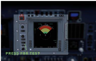
Press once to put radar into Test mode.
