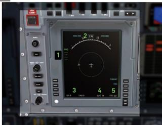
This screen has 2 main functions: Navigation Display (ND) and Engine Information Display. In ND mode, the current flight plan is shown in arc or rose mode, with the heading, distance and ETA (estimated time of arrival) to the next waypoint 1. On the top part, you can also read the current heading and course for the VOR1/ILS 2. On the bottom part, you can read the GS and TAS like on the PFD 3, and also the SAT (Saturated Air Temperature) 4. and TAT (Total Air Temperature) 5.
