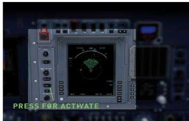
Press again to activate the radar screen and press a third time to close the radar screen.
