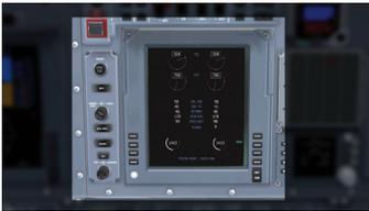
Pressing the ENG button (below the FORMAT button) 9. displays the engine information screen which displays the engine information: TQ is torque, ITT is inter-turbine temperature. You also have information about oil (temperature and quantity), fuel flow, Hydraulics fluid (pressure and quantity) and fuel quantity.
