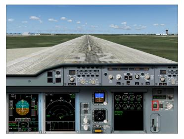
On the large E/WD display (Centre right side - main panel) are displayed the next action that are required to be checked. Each of them are displayed in blue. As soon as the action is performed they disappear.
