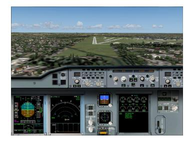
Few seconds before touching the ground, the GPWS voice will announce 'Retard - Retard'. Immediately pull back the throttles to the Idle position. This will disengage the auto-throttle (a sound will warn you).
