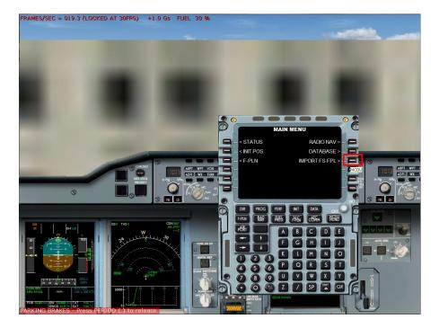
Click with your mouse on RSK3 button "Import FS FPL" (highlighted with a red square on the above picture). This will save the active flight plan into the MCDU. The Flight plan LFBO to LFBP should now appear.
