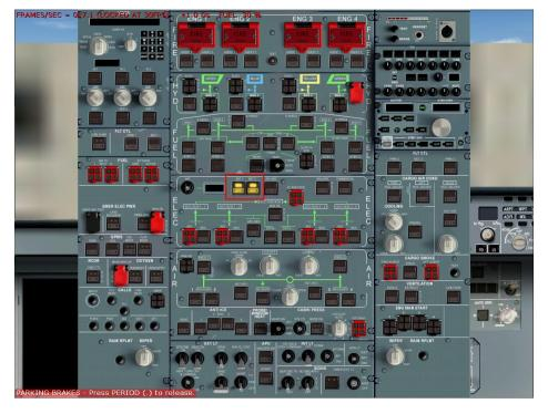
Click on the buttons to switch ON the battery system.
