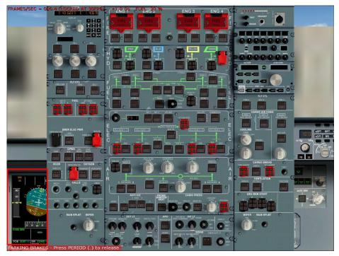
Let's now start the APU (Auxiliary Power Unit). The APU is required to start the engines.
