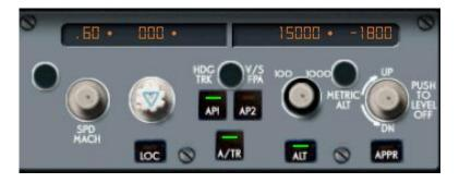
As an example, the data displayed above says that you are flying at Mach 0.60, your heading is  $360^{\circ}$  and you are descending to 15,000 ft with a vertical descent speed of 1,800 ft/minute.
