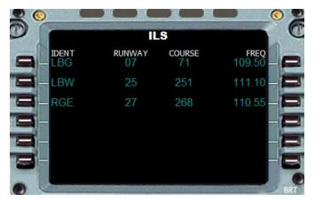
Now, click on one of the buttons located on the right side to select the ATC assigned runway. Today we will be using Runway 07. Press the 109.50 button (RSK1). The ILS frequency is 109.50. This value will be displayed in the lower left corner of the MCDU.
