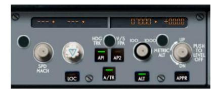
Below is how the MCP should look like when set correctly:
