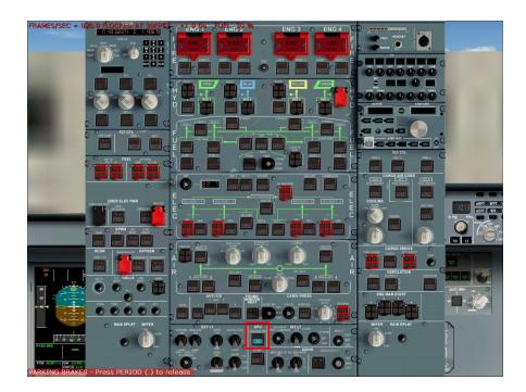
You will hear the APU start and run sound. Wait until the green light AVAIL is ON, confirmed by 'APU AVAIL' shows on the PFD (bottom left pilots side), meaning that APU is ready.
