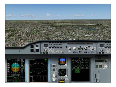
Do not forget to arm spoilers (shift+/ keys) and engage the autobrake. This will be confirmed by the green notes on the E/WD. No blue information should appear on your check-list screen.
