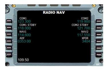
Click on the 3rd left button (LSK3) to enter the frequency into the NAV1 radio.
