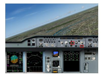
You should now be aligned with the runway. Reduce your speed to 154 Kts, and lower the landing gear.
